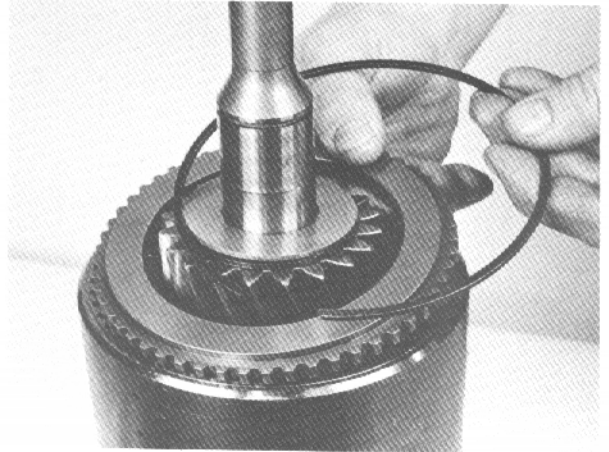
15. Replace the retainer as shown with the recess uppermost and secure with a snap ring.
