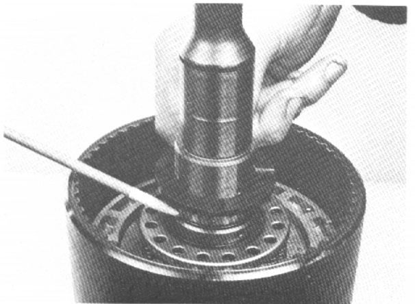
11. Invert shaft, then replace the anti-rotation pin and thrust washer with the oil grooves facing up.
