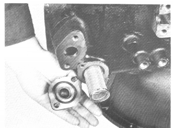
23. Remove the screws, then the oil strainer retaining plate, 'O' ring and oil strainer.
