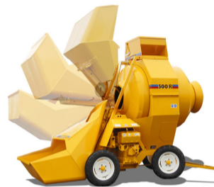
hopper raises hydraulically for drum charging
