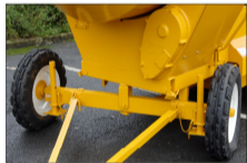
jack-legs are lowered during mixing for stability, swivelling front axle aids site manoeuvrability
