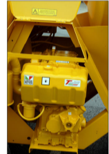
Lister Petter air cooled diesel engine (or 3 phase 415 volt electric motor)
