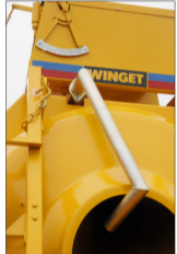
water feed pipe and water tank with calibrated pointer for measured discharge
