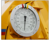
mechanical batchweigher accurate to +/- 3% (optional extra)
