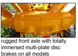
rugged front axle with totally immersed multi-plate disc brakes on all models
