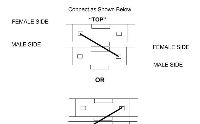
Llink either two diagonal lugs and put power into remaning two lugs
