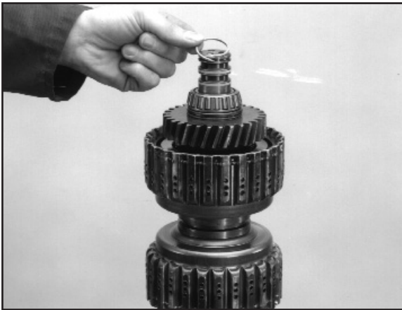
2:2 Remove and discard the 3 sealing rings.
