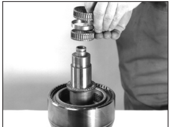
8:6 Remove the needle bearings and spacer.
