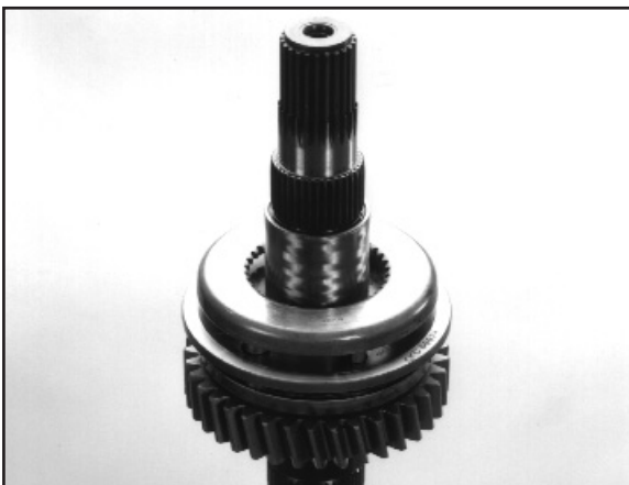
5:16 Replace the 1st / 2nd synchroniser assembly.
