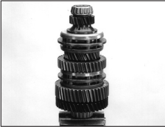
5:1 Position the shaft assembly in a soft jawed vice as shown.
