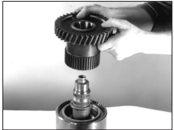
8:5 Remove the 4wd gear.
