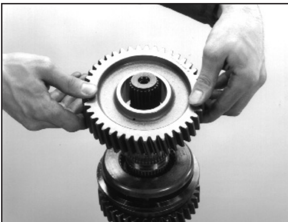
5:9 Remove the 1st gear.
