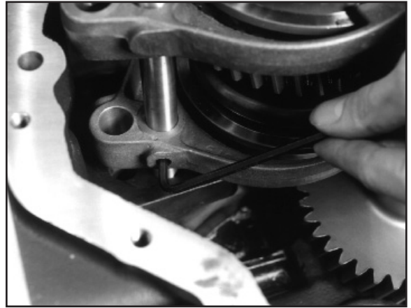
1:16 Remove the 3rd / 4th shift fork screw. Safety Note:- before attempting to remove the 3 / 4th shift rail, replace the detent plug as the ball and spring may shoot out and cause injury.
