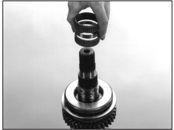
5:10 Remove the needle bearings and spacer.
