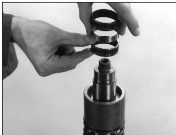
6:6 Remove the two needle bearings and spacer.
