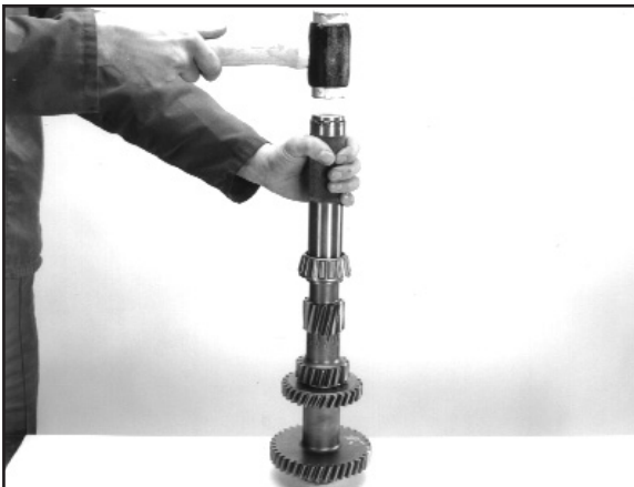
3:3 Using an appropriately sized tube replace the countershaft front and rear bearings.
