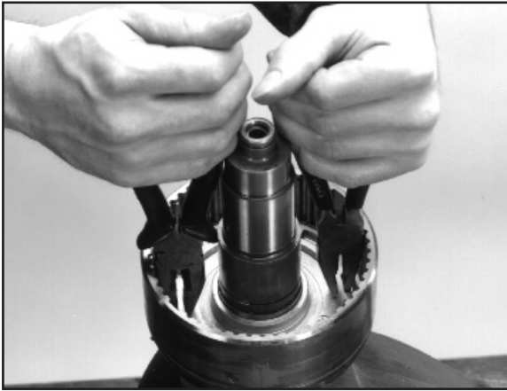
8.13 Remove the piston from the drum.
