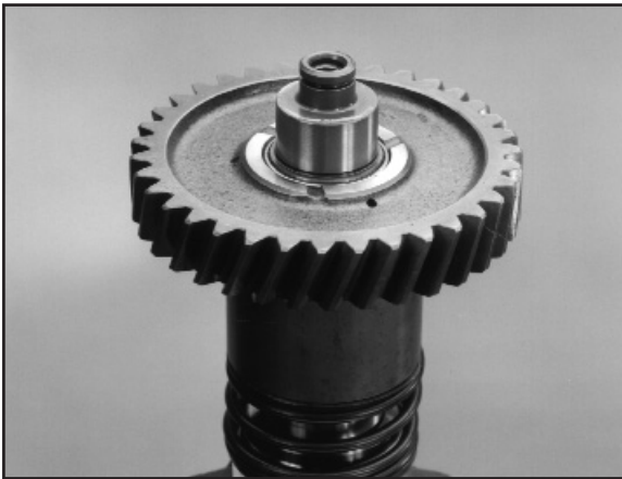
6:20 Replace the 4 wheel drive gear.
