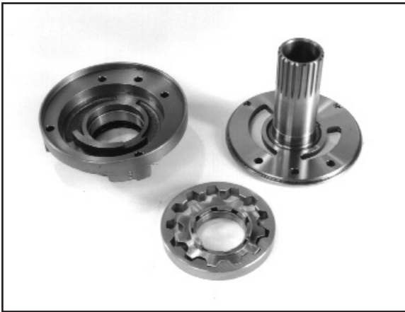
9:1 View showing a dismantled pump assembly.
