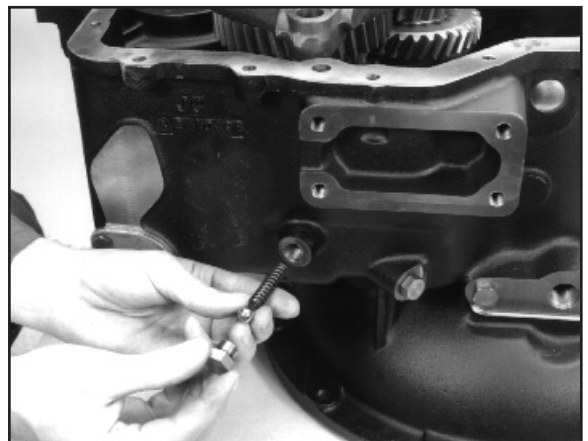
1:18 Remove the detent plug, inner detent ball and spring.
