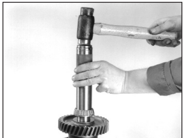
8:27 Using an appropriately sized tube re-fit the rear bearing.
