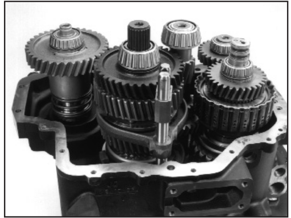
12:14 Rear case with all shaft assemblies fitted.
