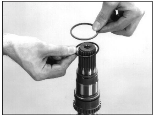
6:11 Remove the piston seal and O ring from the shaft and discard.
