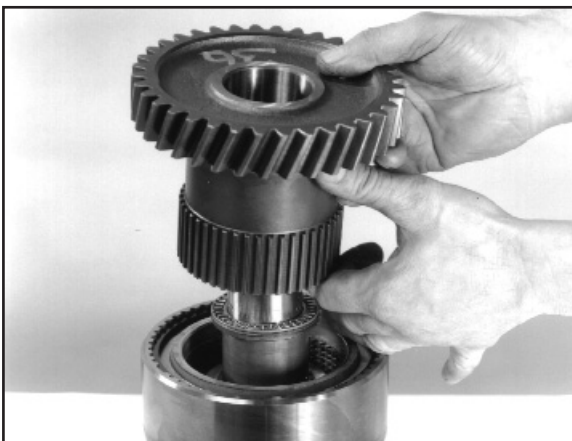
8:24 Refit the 4 wheel drive gear.
