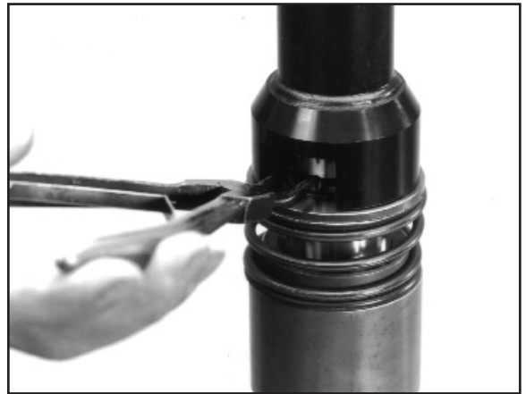
6:17 Using the appropriate tool compress the spring and retainer and refit the circlip. (Tool No.KM3523)
