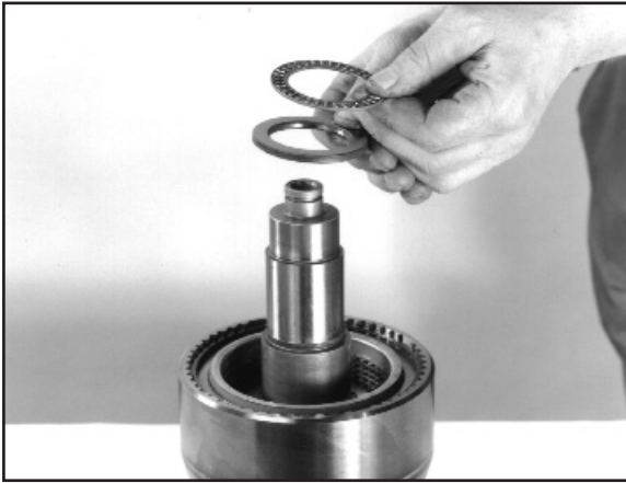
8:7 Remove the needle bearing and thrust washer.
