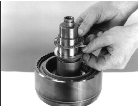
8:23 Refit the thrust washer and needle bearing.
