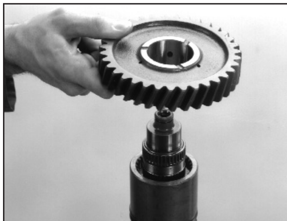
6:5 Remove the 4 wheel drive gear.
