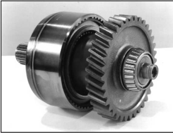
8:1 The hydraulic multi plate clutch 4wd shaft assembly.
