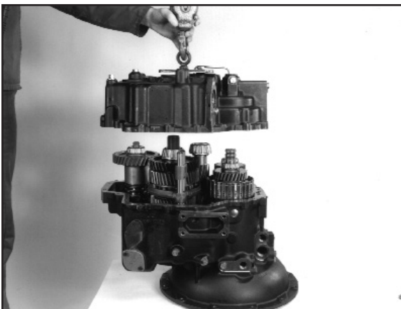
1:9 Remove 17 screws and using a suitable hoist take off the rear transmission case. Lever slots are provided to assist removal.
