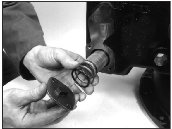
1:23 Remove 2 screws and withdraw the strainer cover, O ring, spacer and strainer.
