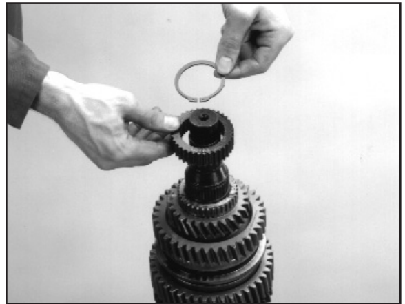
5:5 Remove the circlip and synchro hub.
