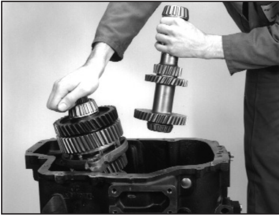
1:19 Remove the counter shaft assembly.
