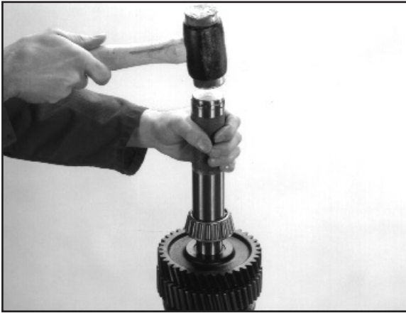
5:20 Using an appropriately sized tube refit the rear bearing.
