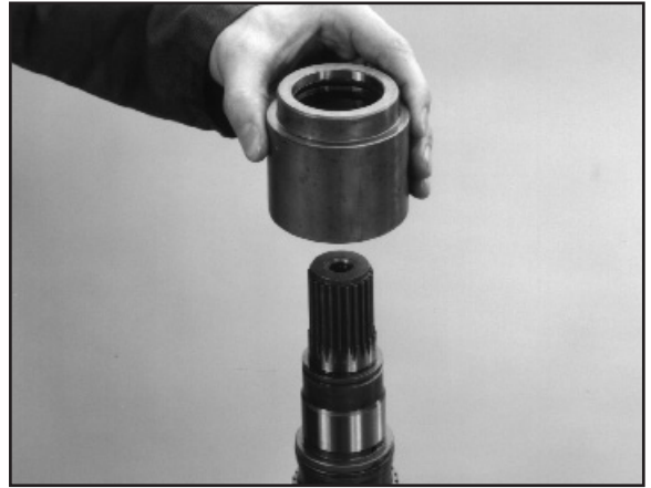
6:10 Remove the piston drum assembly.
