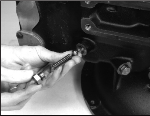
1:13 Remove the outer detent plug , spring and ball.
