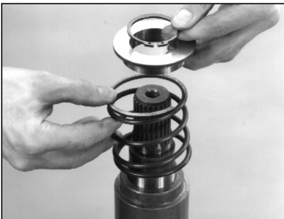
6:9 Remove the circlip, retainer, and spring.
