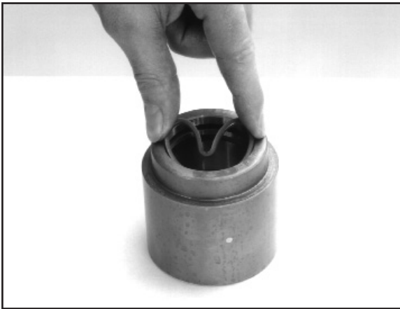
6:14 Fit a new O ring and sealing ring into the piston. Bend the sealing ring into a heart shape as shown to assist assembly.
