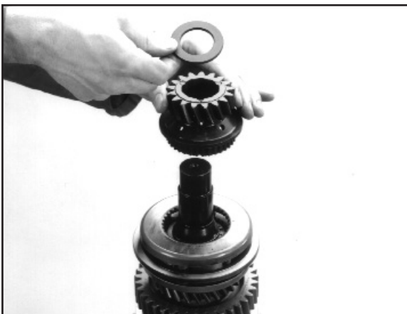
5:3 Remove the thrust washer and 4th gear.
