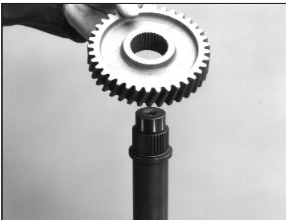
7:3 Remove the 4 wheel drive gear.
