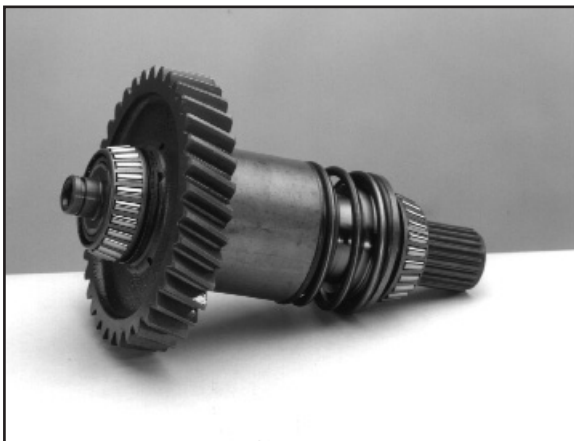
6:1 The hydraulic dog clutch 4 wheel drive assembly.
