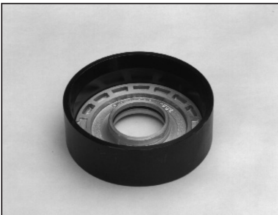
8:18 Using the appropriate tool compress the piston sealing rings. The seals should be left in the tool for a minimum of 30 minutes prior to assembly into the clutch drum. (Tool No.KM3510)
