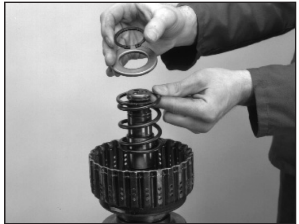
2:11 Remove the circlip, retainer and spring.
