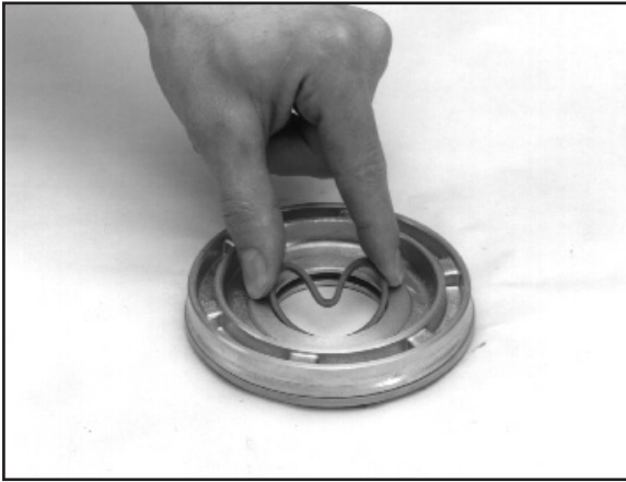
2:15 Re-new the piston sealing rings and O rings. To assist assembly bend the inner sealing ring into a heart shape as shown.
