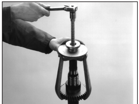
5:12 Using a suitable bearing puller or press. Remove the bearing sleeve , synchro hub and 2nd gear.
