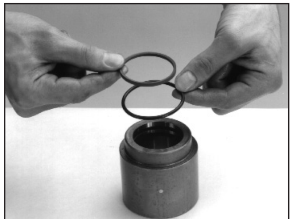
6:12 Remove and discard the piston seal and O ring from the piston drum .
