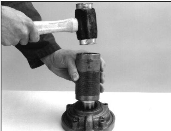
9:2 The pump oil seal may be replaced using an appropriately sized tube.
