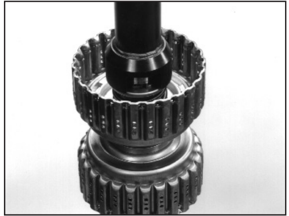
2:18 Using the appropriate tool compress the spring and locate the circlip into its groove. ( Tool No.KM3520)
