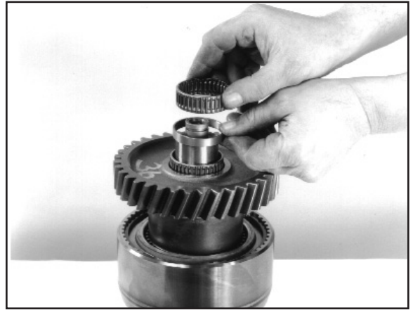
8:25 Refit the needle bearings and spacer.
