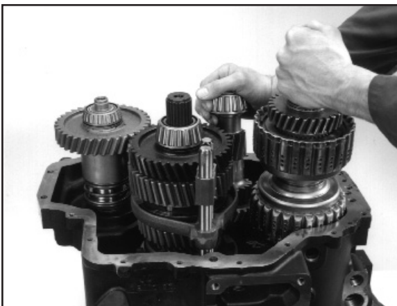
12:13 Lubricate the input shaft front and rear seals with a light grease and re-fit the shaft assembly into the case.
