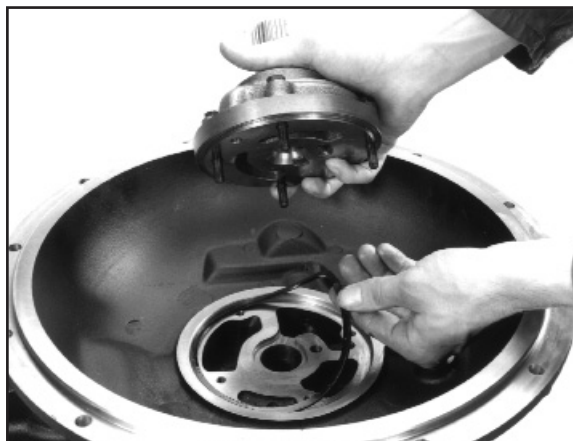
1:29 Invert the case. Remove 4 screws and copper washers then withdraw the pump assembly and sealing ring.
