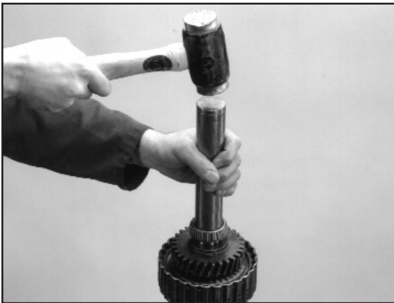
2:23 Using an appropriately sized tube replace the bearing as shown.
