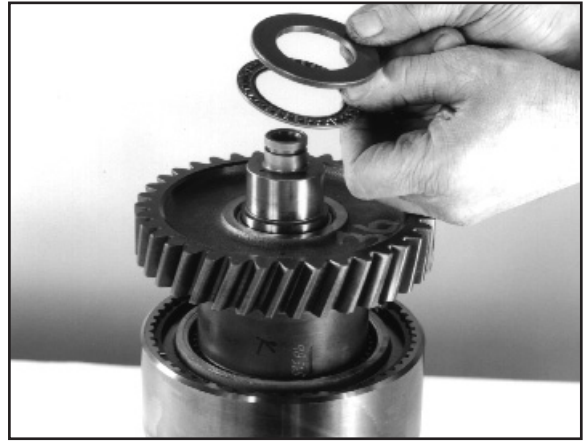
8:4 Remove the thrust washer and needle bearing.
