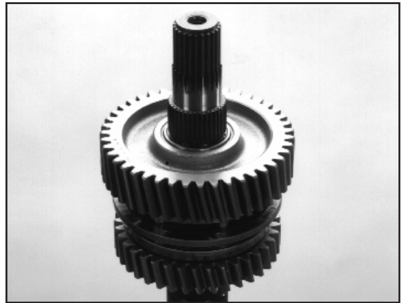
5:18 Replace the 1st gear.
