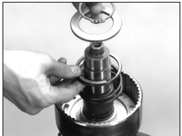
8:12 Remove the clip retainer and spring.
