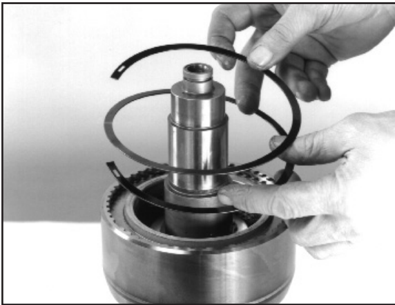
8:8 Remove the clutch pack retaining clip.
