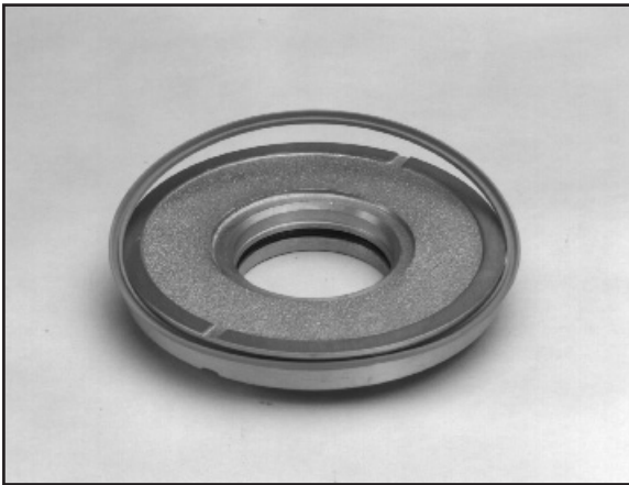
8:17 Re-new the piston sealing rings to assist assembly the seals may be warmed in lukewarm water prior to assembly.
