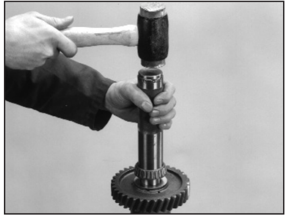
6:22 Using an appropriately sized tube replace the rear bearing.
