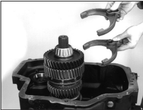
1:20 Remove the 1st / 2nd and 3rd / 4th shift forks.
