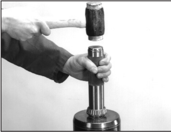
8:16 Using an appropriately sized tube re-fit the front bearing.
