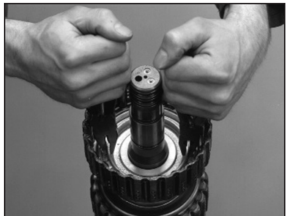
2:12 Using pliers, as shown, pull the piston out of the drum.
