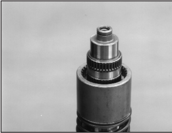
6:19 Invert the shaft and refit the two needle bearings and spacer as shown.
