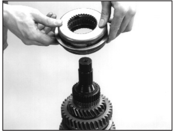
5:4 Remove the 3rd / 4th synchro assembly.
