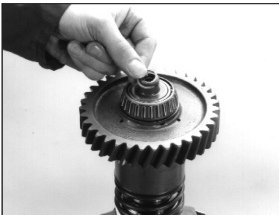
6:2 Position the shaft in a soft jawed vice and remove the sealing ring.
