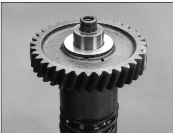
6:21 Replace the thrust washer.
