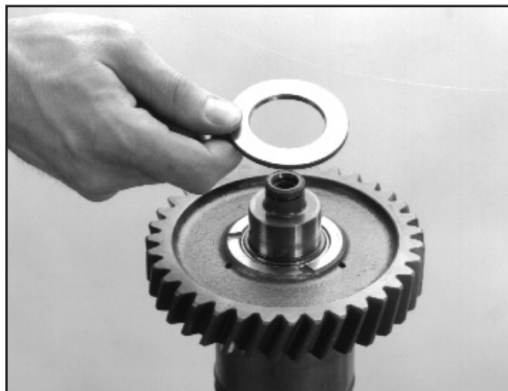
6:4 Remove the thrust washer.
