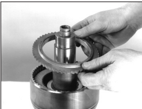
8:9 Remove the clutch pack retaining plate.
