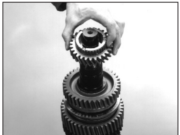
5:6 Remove the 3rd gear.
