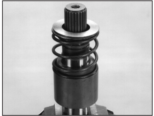
6:16 Replace the piston spring and retainer.
