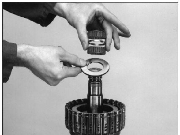
2:6 Remove the bearing, spacer, bearing and thrust washer.
