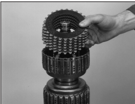
2:9 Remove the clutch pack.
