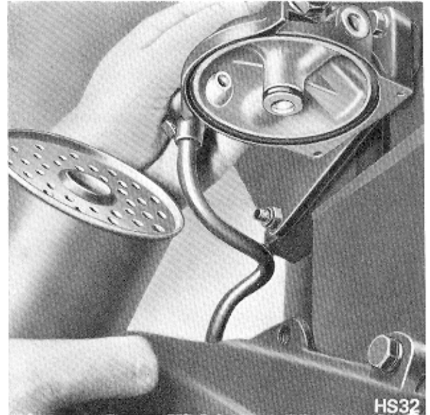
Fig. 21 Changing Fuel Filter
