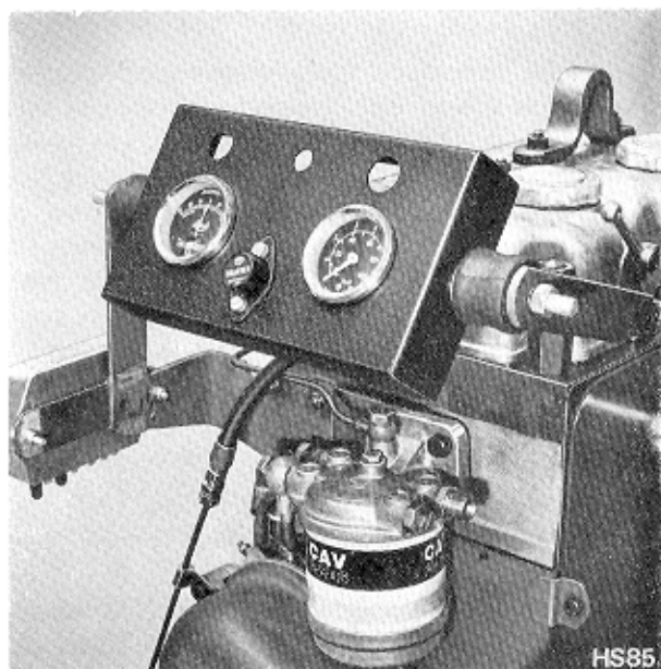
Fig. 145 Gauge Panel with Ammeter and Starter Button
