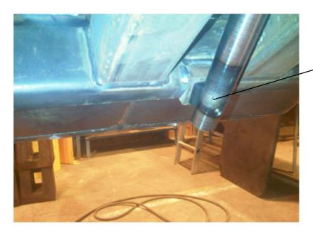
Striker Pin No 555109100, Secure to the Hopper Cradle with one 6S05E Setscrew and one 41S07 Spring Washer, sandwiching the Shim Pack between the Striker Pin and the Hopper Cradle.
