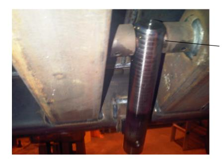
Install the Striker Pin to the underside of the Hopper Cradle. Lubricate the Retaining Pin and Bosses before inserting the Pin into the Hopper Cradle. Secure the Pin using the Grubscrew and tighten. Retaining Pin No 555109300 & Grub Screw No195S03C2
