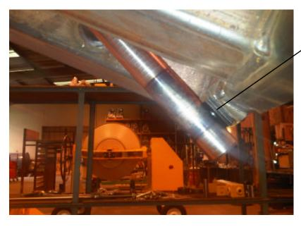
On a 500R insert a full pack of Shims Part No 555109200 between the Striker Pin and Hopper Cradle. On a 300R/400R insert 2 thick shims, 2 medium and 2 thin shims between the Striker Pin and Hopper Cradle. (Part Nos 555109202, 555109203 & 555109204) Sandwich the medium and thin shims between the two thick shims to prevent distortion when the retaining setscrew is tightened.
