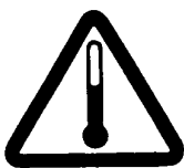
General hot surface warning
