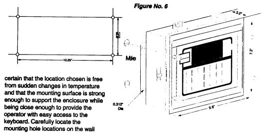
then drill and install the anchor bolts. Attached the enclosure to the wall and securely tighten the retaining bolts.
