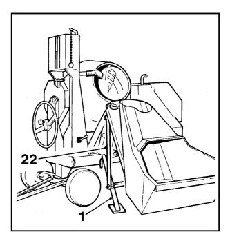
With the lifting equipment, slowly raise the hopper and swing the safety prop (3) up into position. Lower the hopper onto the prop.
