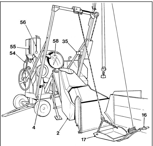
Turn the mixing drum to the MIX position. Allow the mixing to continue for about 1.5 to 2 minutes.
