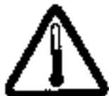
General hot surface warning
