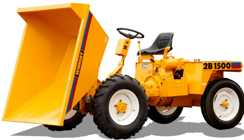
Twin heavy duty tip rams (optional hydraulic tip on 2B1500)
